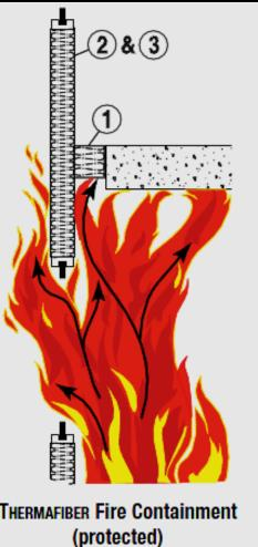
THERMAFIBER Life-Safety Fire Containment Products compartmentalize fire, preventing it from spreading from the floor of origin up to the floor above by:
